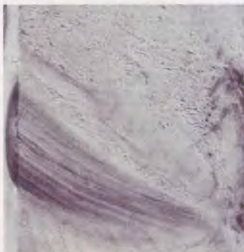
Sound, tight (intergrown), spiked red knot.
